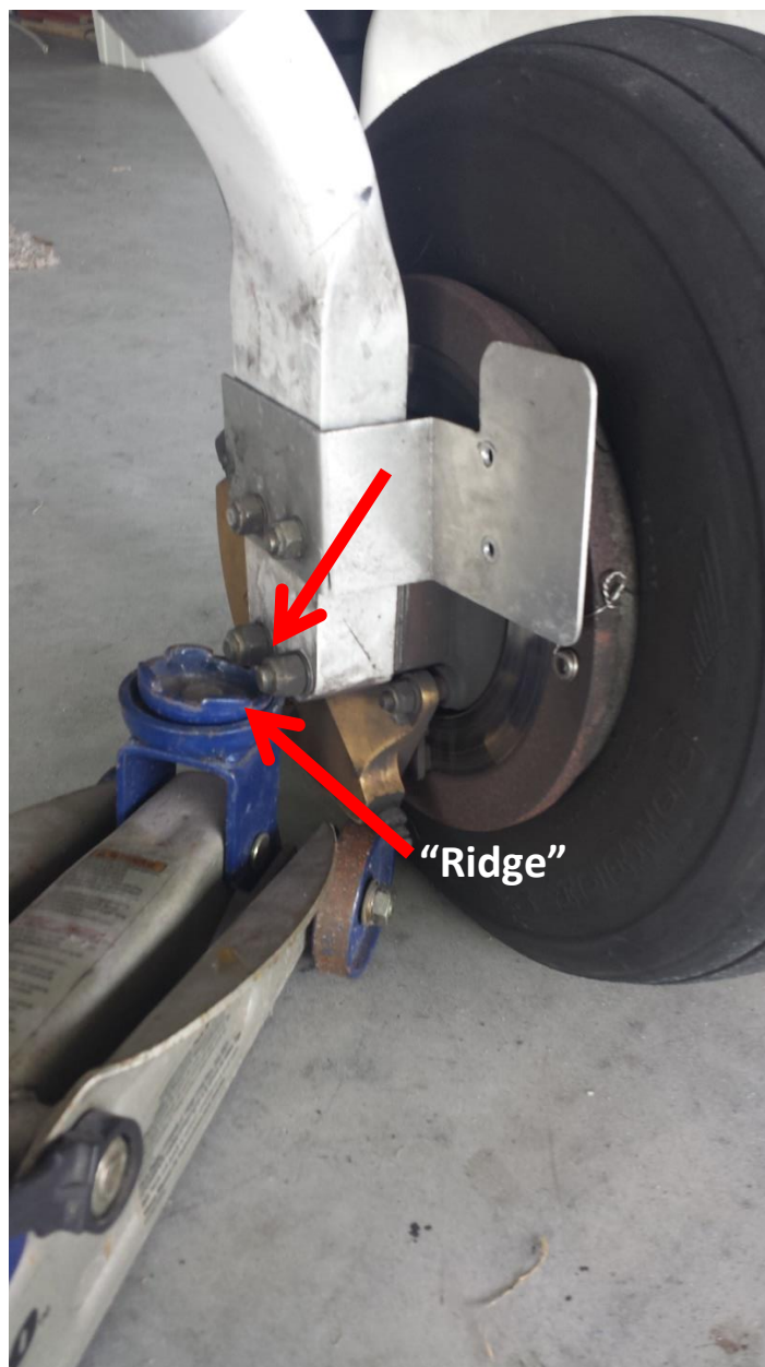
Floor Jack Placement Close Up
