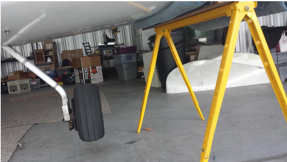
The Saw Horse Supporting the Airplane
