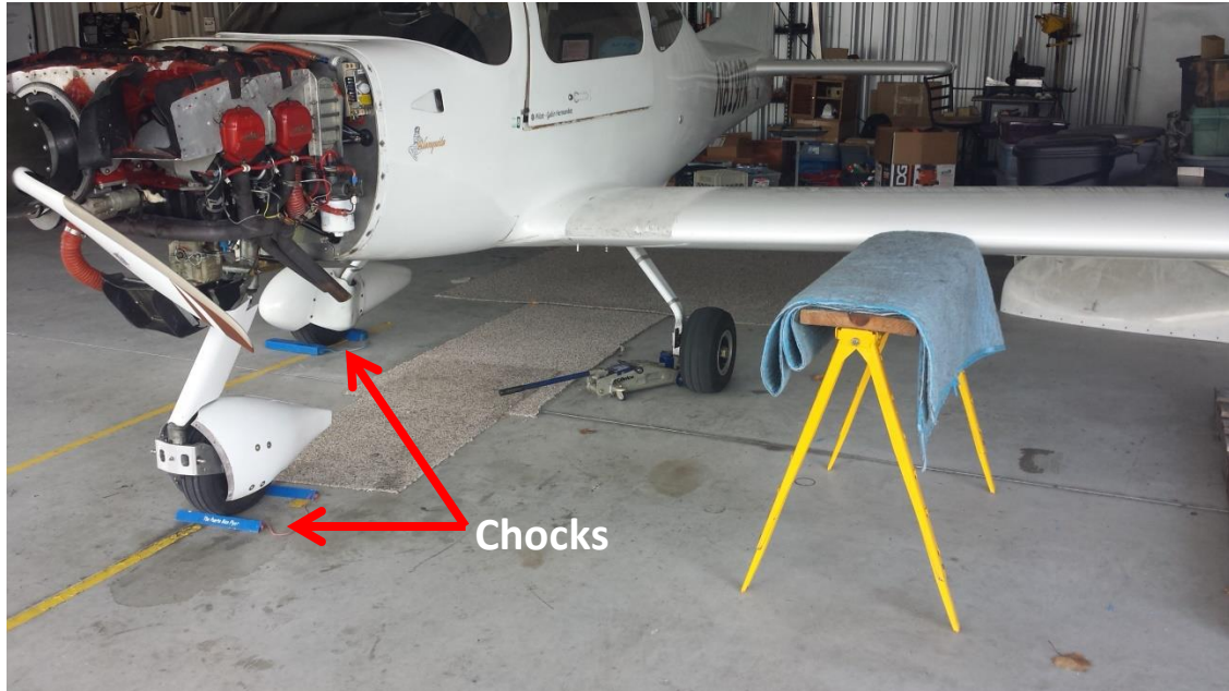
Airplane Chocked With the Floor Jack and Saw Horse in Position
