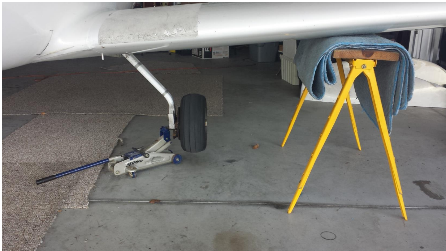
Main Gear Raised and Saw Horse Under the Wing
