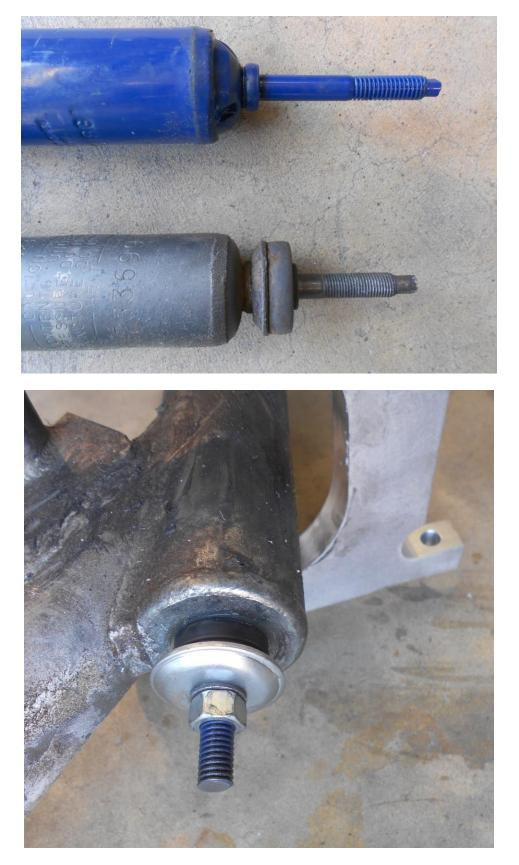
There is a rubber grommet on the bottom of the shock absorber inside the assembly and on the bottom of the entire assembly as seen in the above photos.
