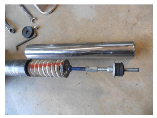
The 3/8" dia. lengthening adaptor threaded rod is shown in detail in the previous photos. The nut provides a stop to help prevent it being over tightened during installation. A rubber grommet is placed there to prevent a metal to metal connection which winds up inside the assembly.
