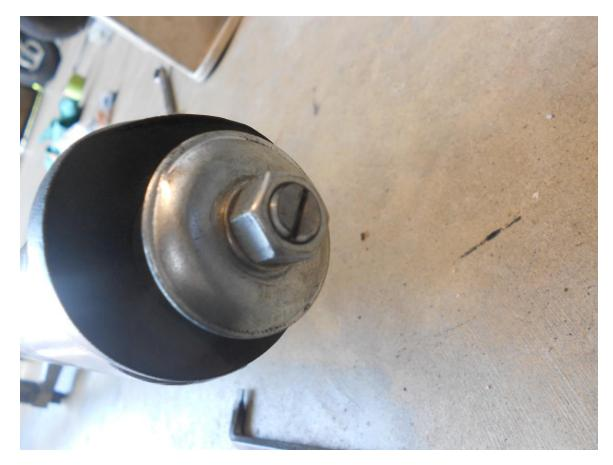
The top of the threaded rod extender needs to have a screwdriver slot cut in to it in order to adjust it during installation.
