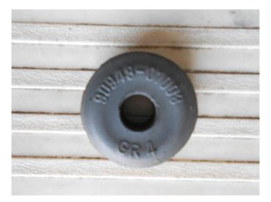
The rubber grommets supplied with the replacement shock absorber were too thick for my particular installation. I would up using a thinner ones (90948-01008) inside the assembly as seen in the above photo.
