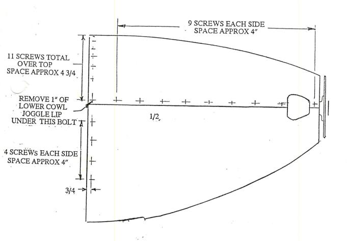
Temporarily assemble the two halves with some #8 bolts and nuts or cleco fasteners along the horizontal parting lines. Locate the holes so they can be used as final screw locations. Carefully remove about 1 inch of the lower cowl joggle lips in the back corners. This will let the upper and lower cowl halves to mate flush in that area. Slip the cowl assembly over the engine. On nose gear aircraft it will be necessary to remove a piece of the lower cowl (about 2 1/2 X 6) to clear the gear.
