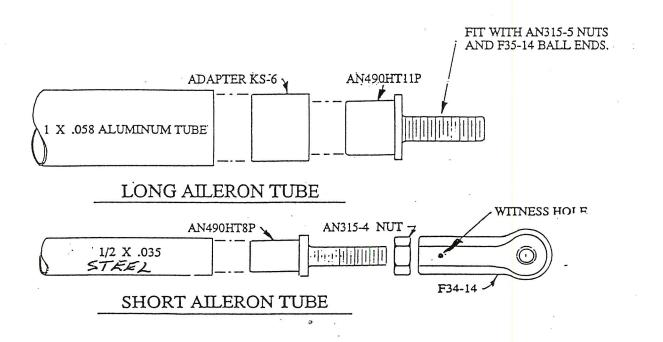
FIGURE - Rod end assemblies for push pull tubes..
