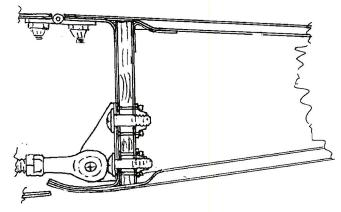
Locate the hinge areas and add a four layer BID prelam 3 inches wide and 10 inches long in each of the two hinge areas per aileron. Lap at least 1 inch up onto the spar surface over this length.
