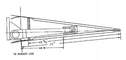
Install the flap track using the supplied flat head 10-32 screws (MS - 24694-556). Tighten screws, but do not bond in place until the location has been verified in final assembly, at which time the tracks may be final adjusted and shimmed to assure proper synchronization between the flaps on both sides, prior to final bonding in place.
