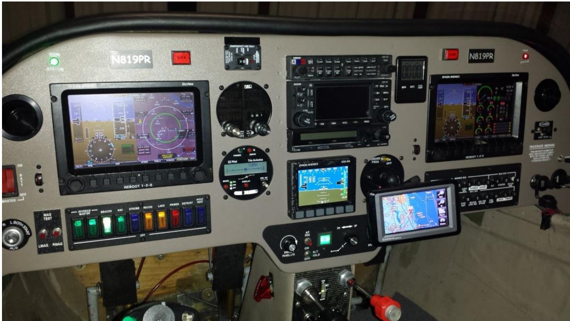
Pilot LED is GREEN while Co-Pilot LED is RED indicating the Pilot controls the trim
