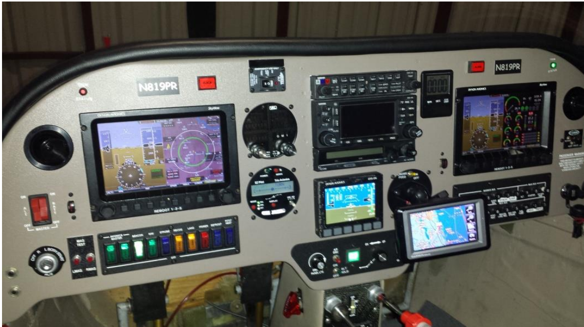
Co-Pilot LED is GREEN while Pilot LED is RED indicating the Co-Pilot controls the trim
