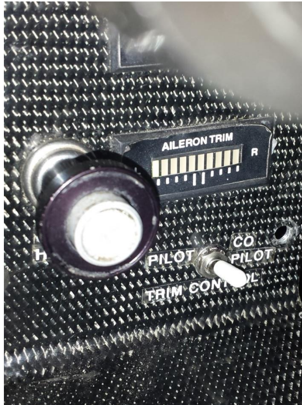
Trim Selector Switch
